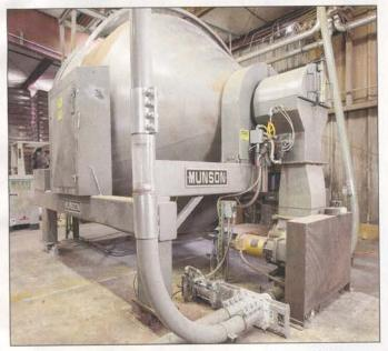
To blend raw material for plywood adhesives at higher rates with greater uniformity, Willamette Valley Company replaced a ribbon blender that agitates material, with a rotary batch mixer that tumbles it.
